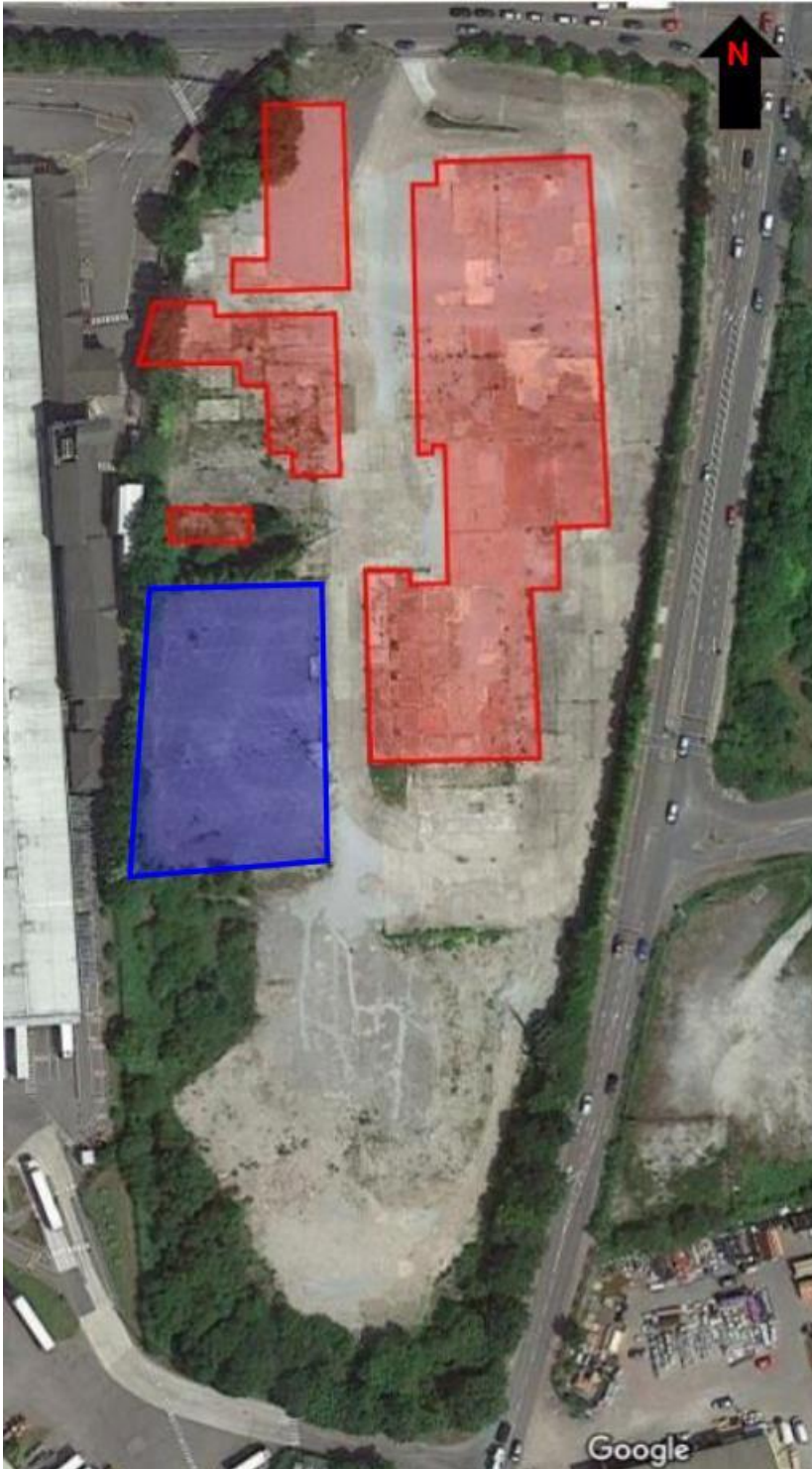
Figure 6: Extract from Google Maps marked up to show existing concrete ground slabs and foundations | red: concrete floor slabs/ foundations, blue: carpark | not to scale
